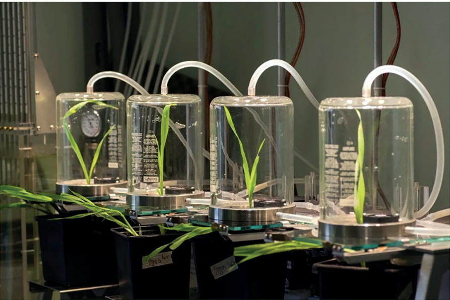
Fig. 11: Jyrkki MAX is a multi-cuvette stationary gas exchange device designed to measure bigger plants like cereals, ferns, tomatoes etc. (Plant Invent Estonia)
