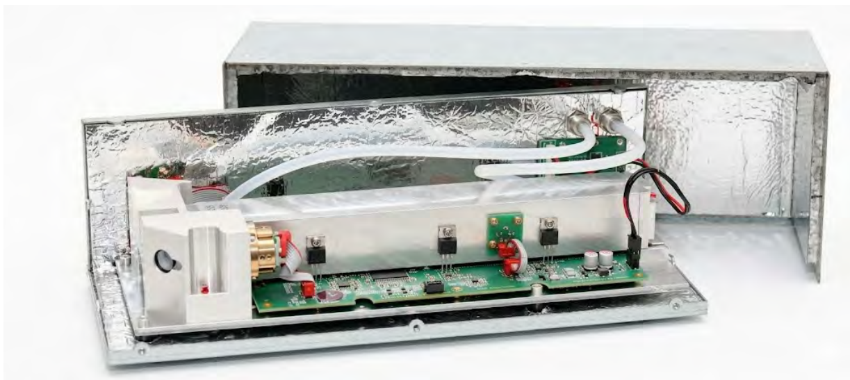
Fig. 5: The SPECTRO.sens optical bench with its associated signal processing electronics, integrated into a thermal housing (Thermobox TBH)
